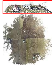
Figure 12.19: Point-cloud generated by the RGB camera mounted on the FW-UAV. The house area shown in the top consists of 163'595 points.
