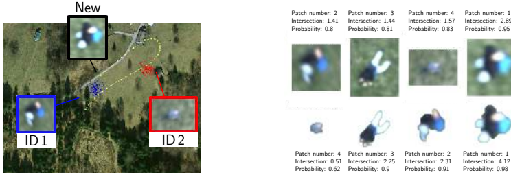
Figure 11.7: Human re-detection: The algorithm needs to decide if the new detection can be associated to an already observed human or if it is, in fact, a new victim. On the right, the histogram similarity is evaluated based on the Intersection metric. The query image is patch number 1.
