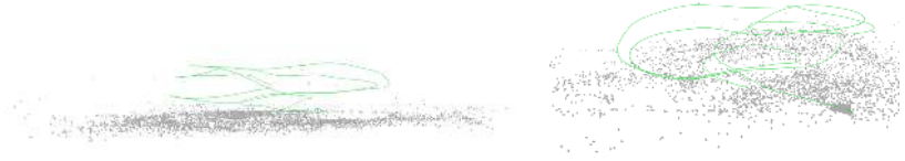
Figure 4.7: Side-view of the generated sparse point-cloud and the estimated trajectory flown by the UAV. The right figure shows take-off and landing spot with increased point-cloud density.
