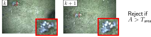
Figure 11.5: Metric outlier rejection: The detection is rejected if the estimated metric area A of the bounding box is above a threshold T_{\text{area}} .
