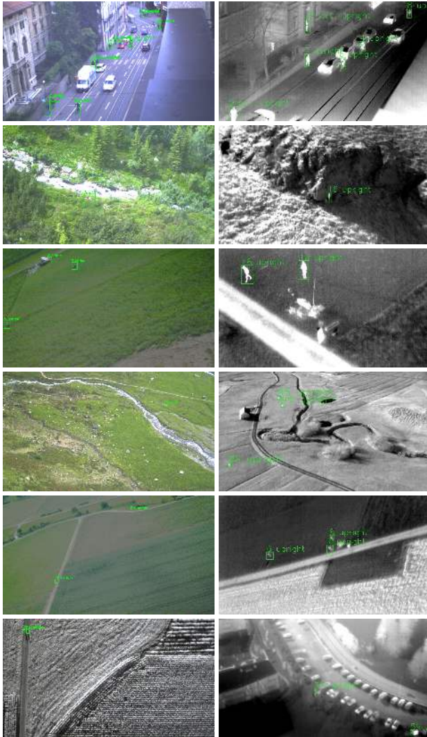
Figure 11.15: Annotated frames of the collected datasets containing a total of over 70 000 humans in different poses, in both optical and thermal imagery, and in a variety of different environments.
