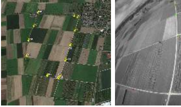
Figure 7.3: Left: Landmark positions in UTM coordinates. Right: Hand-labeled feature positions (green) and reprojected landmark locations (red) given the camera pose estimated by the PNP.
