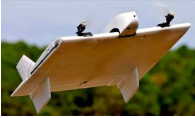
(a) SKATE by Aurora in factory configuration. The head piece contains batteries and two down-looking cameras.
