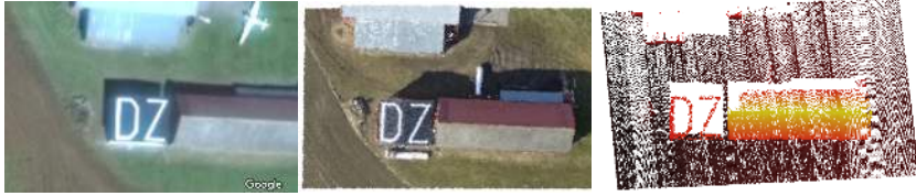
Figure 12.9: Satellite image as reference. Figure 12.10: Vision point-cloud. Figure 12.11: Laser point-cloud colored by height
