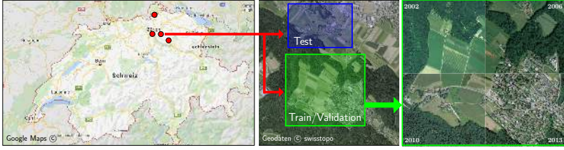
Figure 6.2: From left to right: Four locations in Switzerland are selected to extract training, validation and testing data. Training, validation and testing data is extracted for every location from nearby but non-overlapping areas. Each of these areas consists again of orthoimages and elevation maps of all available years.
