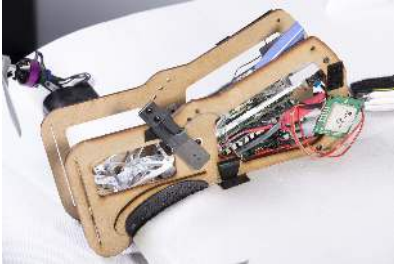
(c) Sensor & processing unit mounted on SKATE. The measurements from the GPS receiver are used to generate a reference trajectory.
