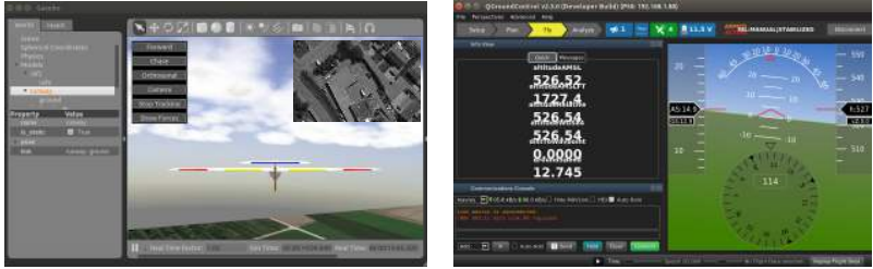
(a) Fixed-wing UAV and synthetic image. (b) Output of QGroundControl in HIL mode.
