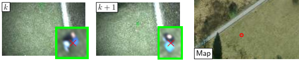
Figure 11.4: Human localization: Based on two subsequent detections, the geo-referenced human position can be triangulated, as visualized in the satellite orthoimage.
